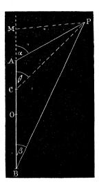
Let A B be the axis of the coil, so that A and B are the centres of its two faces; then A B=2f. Let O be the middle point of A B. Let P be the attracted point, P M its perpendicular distance p from A B. Let P A M= $\alpha$ , P B M= $\beta$ .
